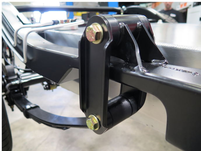
Tri-Five Install Shackles_IMG_2030.jpg
