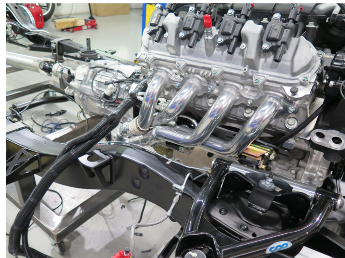
Tri-Five Install LT Headers_IMG_2762.jpg
