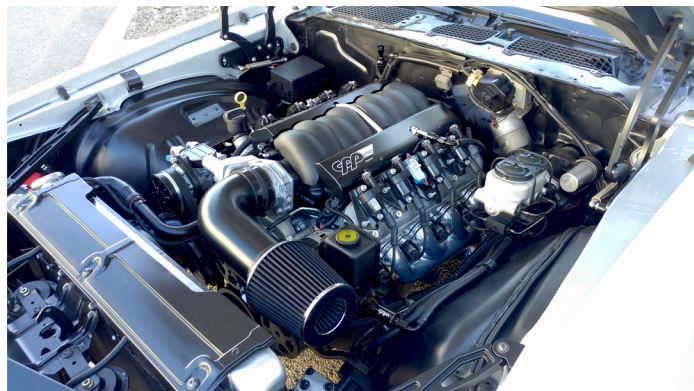
70-Camaro-LS Engine install.jpg
