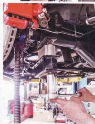
**04-06** Regardless of whether you're just swapping out coils and shocks or upgrading with the complete kit, do not crack a single nut loose until your rearend's safely and securely supported—separately from the chassis, as you'll need to allow room for parts removal articulation.
