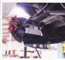
13 When assembling the new lower coilover shock mount, make sure the bracket's built-in stud angle is orientated correctly (pointing downward).
