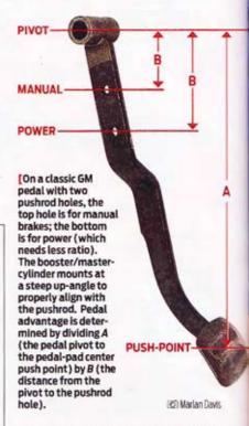
In any event, don't compromise safety. If the pedal/pushrod stroke ends up too short to allow the master cylinder's full piston travel, full system pressure cannot be achieved. Conversely, if the stroke is too long, the brakes could go into bind and lock up. In no circumstances should you permit the brake pedal to go over center.
