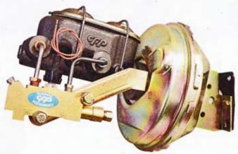
This Classic Performance Products (CPP) power booster, dual master cylinder, and proportioning valve combo is representative of the OE power-brake system used on most classic 1967-and-later GM vehicles. The rear bracket bolts to the vertical firewall and angles the unit up about 17 degrees. CPP offers many variations, including retrofit kits for earlier vehicles.
