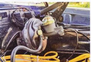
[This 1966 GTO is still equipped with only a single-pot master cylinder with optional power booster; it also has the up-angle needed to connect properly to the pedal's lower hole. Dual masters were Federally mandated beginning in 1967, and are a great safety enhancement for earlier cars.
