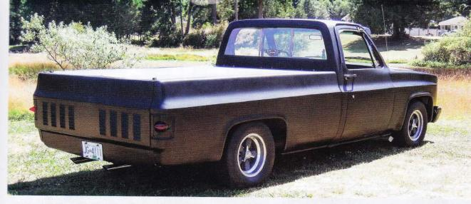
While the Chevy retains its stock 350, it's Quadrajet (Q-Jet) four-barrel carburetor, new headers and other dress-up additions keep it running right and looking clean. The new Saginaw four-speed transmission gives Bob a quality setup that keeps the wheels turning. Eaton 4.11 posi increases
