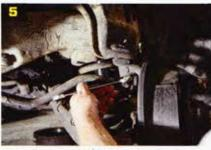
After jacking up the car and placing it on jack stands, we removed the original 14x5 steel wheels. These will no longer fit due to the disc brakes so they will be going to the swap meet oile.
