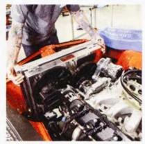
As the sun was setting on Day 2 we were installing the Holley Frostbite three-row, dual pass LS swap radiator. This piece came ready to go with both the inlet and outlet built on the passenger side and provisions for the LS head steam port plumbing. To move tons of air we added a Derale shroud and twin-fan kit to the mix.
