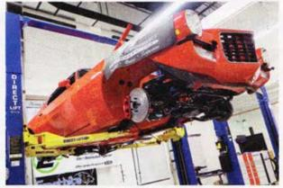
By the end of Day 1, we had the Camaro stripped down and all of the CPP suspension installed under the car. The front kit included CPP's tubular control arms and their badass spindles that utilize C7 Corvette sealed bearing hubs, which are quite a bit stronger than the C6 hubs used in many kits. The front 13-inch rotors came slotted, drilled, and zinc washed.
