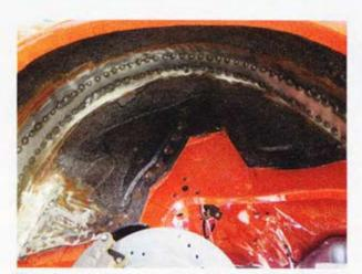
We had seven days to get our rebuild done so we decided to spend a long day before the official start knocking out the Classic Performance Products (CPP) wide wheeltub kit. In short, the inner rear wheelhouse is cut out, moved inboard, and then the resulting gap is bridged with a slick piece from CPP. This, along with a few other parts, will let us run the massive 315/30R18 RT615K+ Falken tires. With that completed, one day was gone with six to go.
