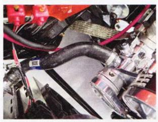
We've done enough of these builds that we have a pretty good idea of what radiator hoses will work with minimal modifications. We also dropped in the Optima YellowTop battery and finished up the wiring, including the rather large, 240-amp, braided ground strap from Painless Performance.
