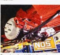
To replace the old 1D-bolt peg-leg rear, CPP supplied a complete 9-inch rear filled with 3.70 gears and a Detroit Truetrac posi. The rear came with the 12-inch disc brake system already installed, which was a real time saver. You can also spy CPP's narrow leaf springs. When combined with their shackle kit, the system will give us just enough room for the 315mm rear tires.
