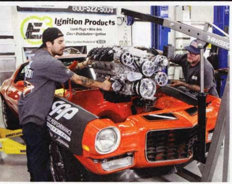
Before lunch on Day 2, we dropped the new SDPC Chevrolet Performance LS crate engine into the Camaro, which gave us the warm, fuzzy feeling that we were ahead of the game. Before the build we dyno-tested the engine at Westech Performance and it churned out 540 hp NA and 660 hp with a nitrous hit.
