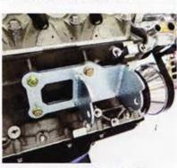
Next up was bolting the Holley LS engine mount plates to the LS block. The Holley LS swap parts, when used together, ensure that the headers clear properly and that the right driveline angle is achieved.
