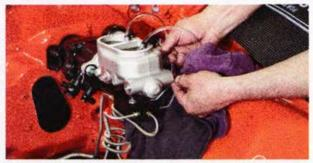
The crew from CPP also got busy installing and bleeding their Hydra Stop braking system. The Hydra Stop uses fluid pressure from the power steering pump to provide braking assist.
