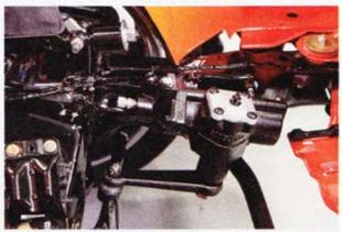
CPP also finished up the Camaro's steering system by installing their 500 steering gear box. The box features a 14.7:1 ratio that's fast for quick maneuvers, but not so fast that it feels twitchy cruising down the highway.
