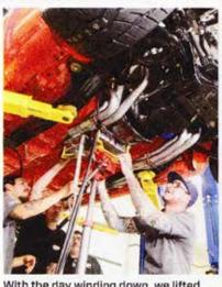
With the day winding down, we lifted the Performance Automatic 4L70E into place and bolted it in using the Holley LS swap transmission brace and an Energy Suspension poly trans mount. We called Day 2 a wrap since we were pretty happy with what we had done in the first two days of the week.
