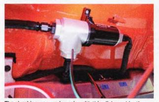
The plumbing was made easier with this slick combination fuel filter and regulator from Holley. As implied, the regulator has an integral, fully serviceable fuel filter. This saves space and money since less fittings are needed to plumb it all in. The regulator itself came preset at the required 59.5 psi needed by most LS EFI systems.
