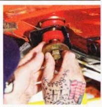
The chassis upgrade also included swapping to Energy Suspension polyurethane subframe bushings and fresh Grade 8 hardware. The poly bushings will firm up the chassis without being overly harsh like solid mounts.
