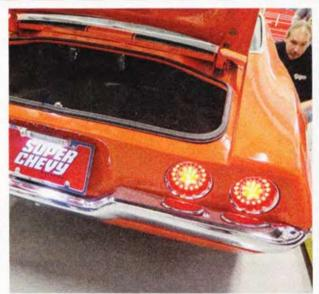
The guys from United Pacific also stopped by with a complete LED lighting kit for our Camaro. We opted to ditch the backup lights in the taillights and have two pairs of brake lights with an attention-grabbing sequential module. To make up for losing the reverse lights we added a very cool license plate frame, also from United Pacific, which incorporated a plate light and very bright LED reverse lights. Day 3 and most of Day 4 were spent wiring up the Camaro.
