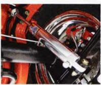
Using CPPs kit, the rear shocks were moved inboard of the frameralls for more tire clearance and were set up to no longer be staggered. The double-adjustable billet shocks will let us easily tune for different driving events. The front system received double-adjustable collovers to give us a ton of tuning options.
