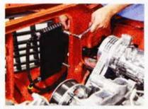
Next up, we were able to install the transmission cooler from Performance Automatic on the front of the core support using some standoffs that Jason knocked out in our fab room.
