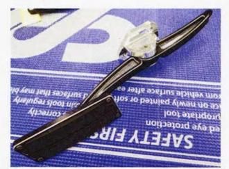
This beautiful gas pedal assembly came from Clayton Machine Works and is almost too nice to stomp on, but we will. The kit also came with a matching brake pedal pad.
