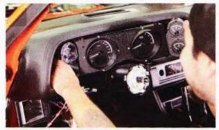
With the column installed we could slide in the new Dakota Digital HDX gauge cluster. The new HDX line is pretty sweet in that it can be configured in a host of different colors either on the dash itself or by way of a smartphone, app, and Bluetooth connection! The HDX utilizes the stock OE bezel for a factory, yet upgraded, look.
