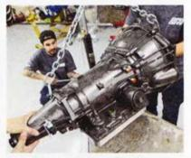
As darkness fell, we readied the Performance Automatic PAGM Street Smart 4L70E four-speed overdrive transmission for its installation. The 4L70E came fully upgraded with improved clutches, a modified valvebody, and other upgrades to play well with our LS376 engine. In fact, it was specifically designed to work with our LS376/515 crate engine.
