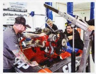
Day 1 of the official build started off with a complete teardown of the Camaro. The drivetrain along will all of the suspension and wiring was yanked so we could get busy installing the new parts.
