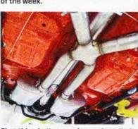
First thing in the morning we installed the fresh-off-the-balancer 3.5-inch aluminum driveshaft from Inland Empire Driveline and started hanging the Hooker Blackheart stainless 2.5-inch exhaust system using the Hooker adapters to step up to the 3-inch collectors on our headers.
