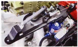
The throttle cable from the Clayton Machine Works pedal was run to the Holley Terminator and hooked up just like any carburetor would be. You can also spot the nitrous solenoid for our NOS Cheater system. Why? Because a little more power is almost just enough.
