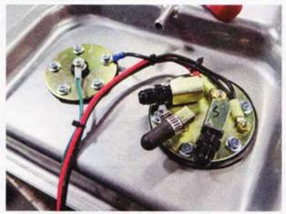
Day 2 started with tackling the new EFI fuel system. First up was the Holley Sniper second-gen Camaro gas tank. It came fully baffled with a 255-lph internal fuel pump. The tank itself was silver powdercoated and included straps and the required sending unit.
