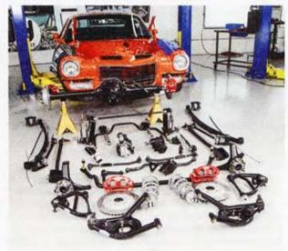
The first new parts to go on were the suspension, braking, and steering parts from CPP. This kit is a lot like their PTK4 offering, but with a few upgrades and a couple of new items such as the subframe connectors and shock relocating system.
