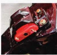
The Holley engine mount plates were designed to work with the secondgen Camaro's clamshell-style engine mounts. We ditched the squishy rubber bushings in the mounts and replaced them with Energy Suspension polyurethane pieces.
