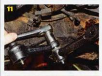
Our 1964 Chevelle originally had 13/16-inch pilot holes for the steering linkage, while 1965-'67 featured 7/8-inch holes. The CPP kit (PN 6467SLK-CP) includes the pitman arm, idler arm, centerlink, inner tie rods, outer tie rods, and billet sleeves. Chevrolet went back to the 13/16-inch equipment for 1968-'72, but the centerlink is 3/4-inch wider. We are replacing the entire steering assembly so 7/8-inch is fine with us.
