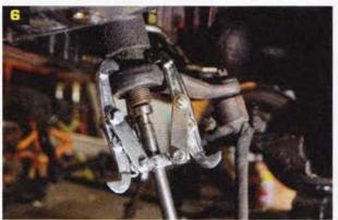
After jacking up the Chevelle we secured it on jack stands and started the disassembly process. The cotter pin on the outer tie-rod ends are removed and we loosen the castle nut with an 11/16-inch wrench.
