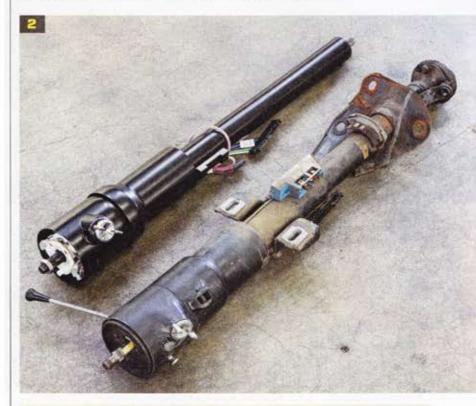
Ididit wrote the book on retrofit tilt steering columns for the Chevrolet Chevelle, Camaro, and Nova, among many others. We're not surprised by this latest innovation from ididit: a bolt-in, factory-style steering column that includes the locking Ignition switch and all of the electrics.
